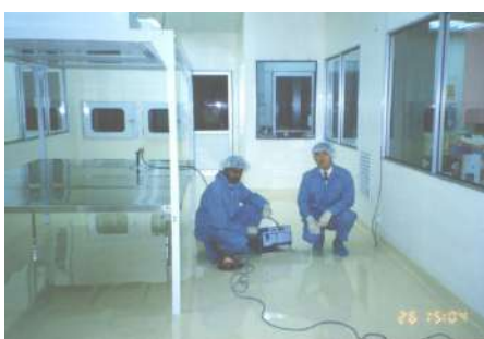
Testing of Fed Std Class 10K Cleanroom
